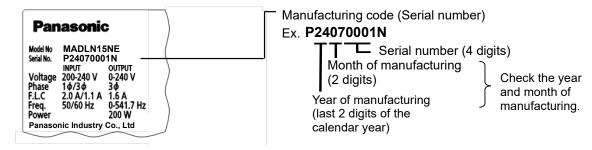
The manufacturing code (serial number) shown on the label attached to the front surface of the package box follows the following rule.
