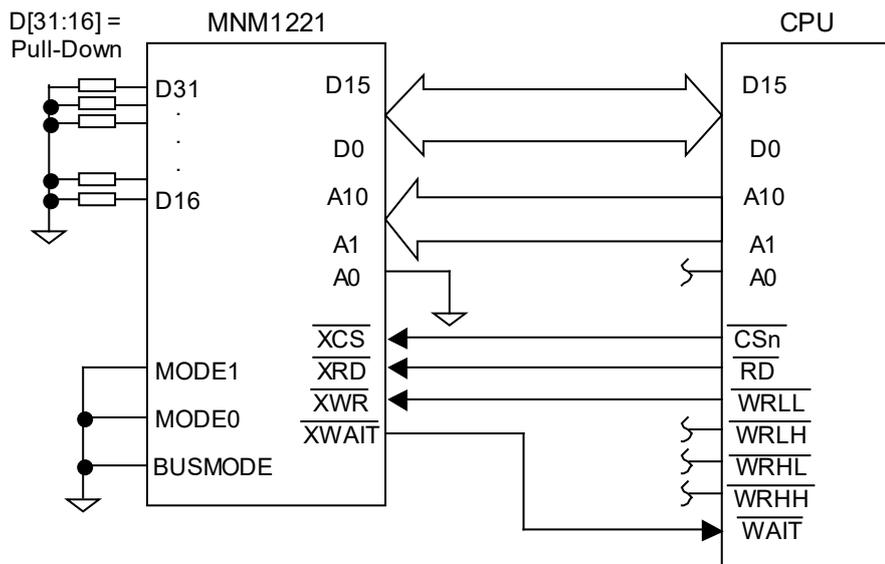
Note: Approximately 10 k Ohm is suitable for the pull-down registers on D[31:16].
