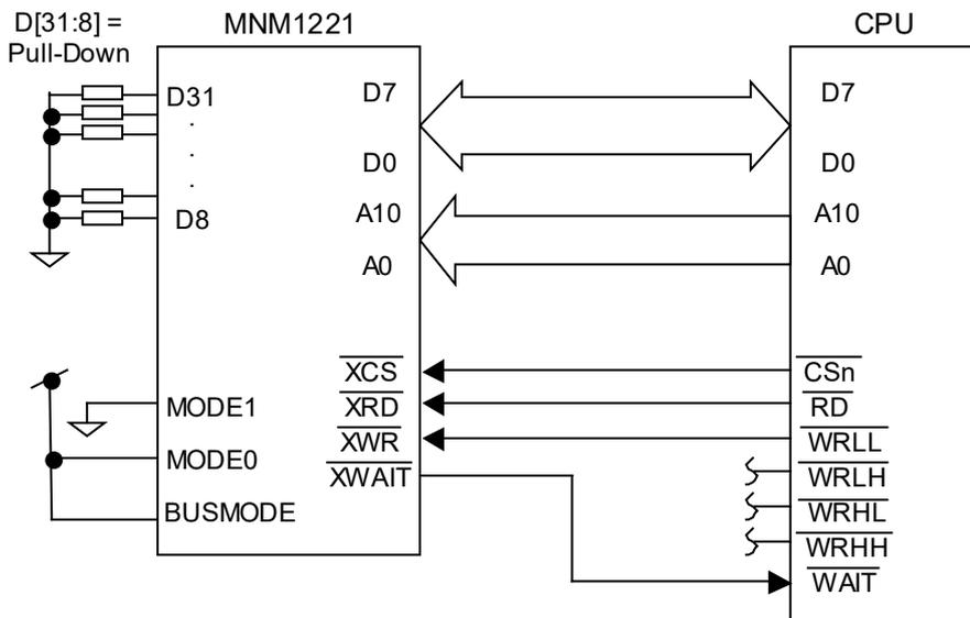
Note: For pull-down resistor for unused data-bus, about 10 k Ohm is recommended.
